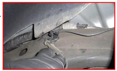
Remove the brake line bracket on the differential.
