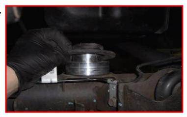
Install the springs back into the vehicle. Raise the axle up to hold the springs in place.
