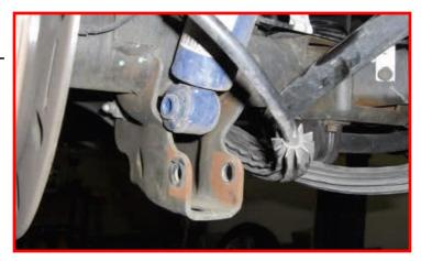
Remove the lower sway bar end link from the sway bar. Let hang out of the way.
