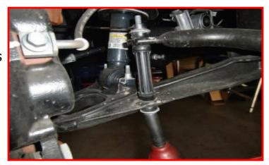
Jounce the vehicle to get it to settle to the new ride height. Once this is done, torque the upper control arm hardware to 120 ft-lbs (final torque to be done by the alignment tech), the lower control arm hardware to 150 ft-lbs, and upper strut hardware to 30 ft-lbs.
