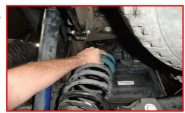
Place the ReadyLIFT spacer onto the axle. Install the rubber spring isolator onto the spacer.
