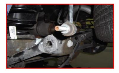
Reconnect the lower shock using the factory hardware. Do not tighten at this time.
