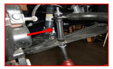
Loosen but do not remove the upper ball joint.
