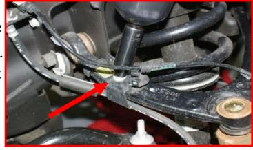
Remove the sway bar end links from the lower control arm. Let the sway bar hang out of the way.
