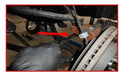
Strike the upper ball joint boss on the knuckle with a dead blow hammer to dislodge the taper. Disconnect the upper ball joint completely and let the knuckle hang out of the way. Make sure to not over extend the brake/ABS lines. Adjust as necessary.
