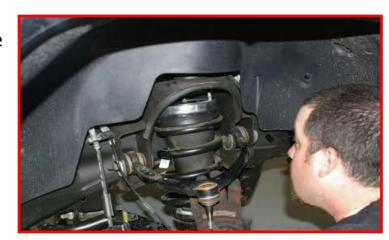
Install the lower ReadyLIFT strut spacer between the strut cross pin and the lower control arm using the factory hardware. Torque to 35 ft-lbs.
