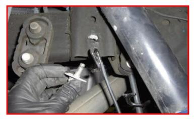
Support the axle with a suitable jack. Remove the lower shock mount from the axle.
