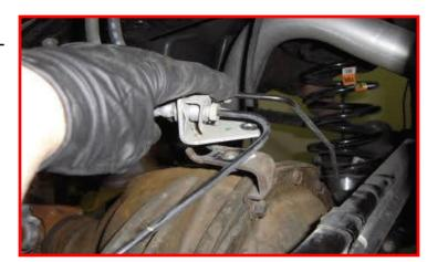
Remove the parking brake bracket on the frame rail. Let hang out of the way.
