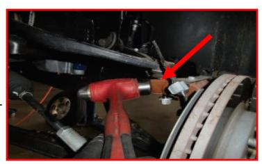
Support the lower control arm with a suitable jack, remove the lower strut hardware. Loosen but do not remove the lower control arm hardware at the frame.
