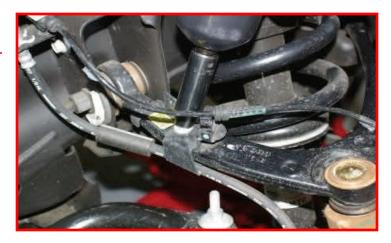
Install the sway bar end links. Torque to 15 ft-lbs. Install the wheels and lower the vehicle to the ground. Torque the lug nuts to the wheel manufacturer's specs.
