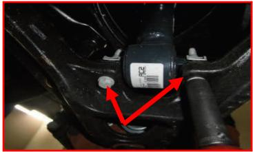
Remove all electrical harness clips on the top of the upper strut studs. Magna-ride vehicles disconnect the electrical connector attached to the strut. Remove the upper strut hardware. Remove the strut from the vehicle.
