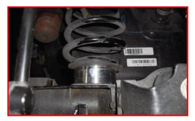
Reinstall the sway bar end link using the factory hardware. Torque to 30 ft-lbs.
