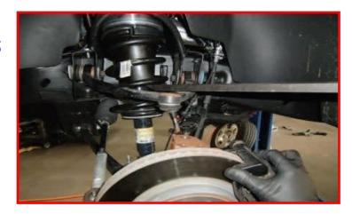
Install the brake line/ ABS bracket to the upper control arm using the factory hardware. Torque to 5 ft-lbs.
